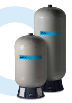
The MixMaster™ series of composite baffle tanks are a superior alternative to traditional contact tanks found in many water treatment systems. MixMaster tanks utilize a patented internal baffle and diffuser system that redirects the treated water through a series of internal chambers. This unique baffle design creates turbulence which boosts the mixing of water and injected disinfectants such as chlorine or ozone, while nearly quadrupling the contact time compared with a standard contact tank.
