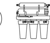
The OneStop+^{\mbox{\tiny TM}} system provides protection from scale formation on internal and external plumbing surfaces. Additionally, it reduces heavy metals such as copper, lead, mercury, zinc and cadmium. It can be installed at the point of entry to a building to treat both hot and cold water, or it can be located directly before a water heater, boiler, or other water using device that requires protection from hard water.
