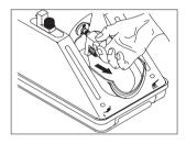
Press the green release button and pull off the basic adaptor. Keep the adaptor in the recess.
